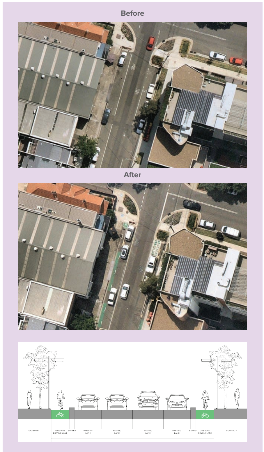
(Figure 39) Example of parking protect bicycle lane at Dunning Avenue, Sydney. A way to make riding easy. Source: Aerial images sourced from Nearmap, cross-section image by CrossleyTP.
