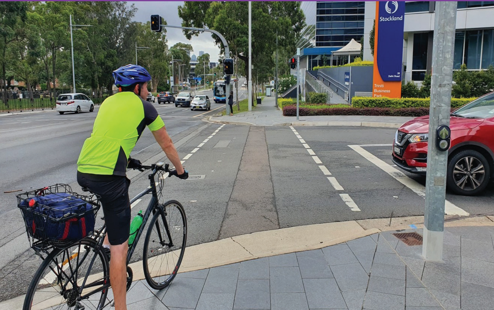
Figure 33 – Delhi Road, North Ryde. Adding bicycle lanterns will make it legal for people riding on shared user paths to cross at signalised intersections.
