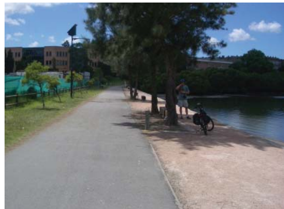
Gravel Pavement Stabilised decomposed granite provides additional trafficable area along main pathway (Meadowbank, Ryde)
