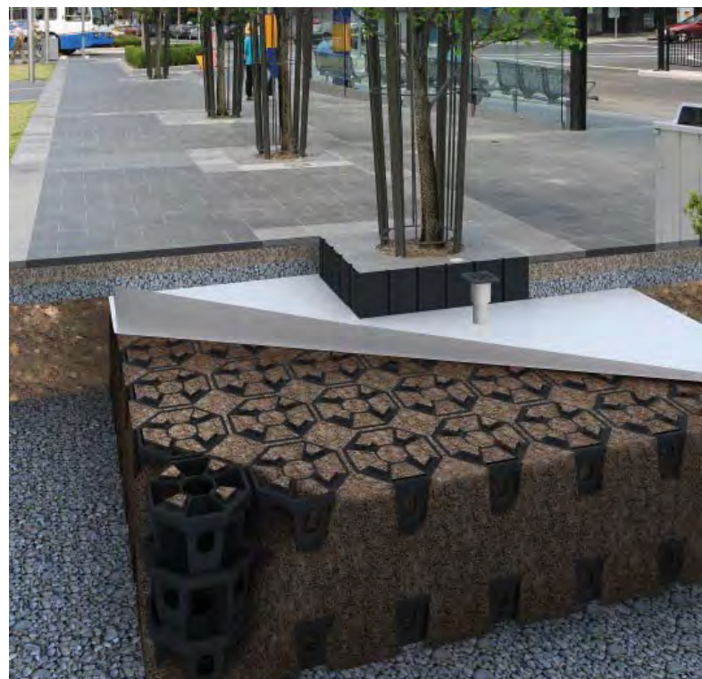
As an alternative to the basalt gap graded structural soil, there are some proprietary systems such as Citygreen that rely on plastic high density grates to support the soil.
