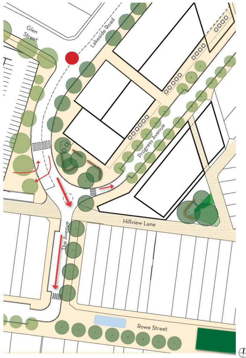
Above: Detail plan illustrating option 1, including one way access - southbound on The Avenue, relocation of the roundabout from The Avenue and Hillview lane intersection to Lakeside Road and Glen Street Reserve.
