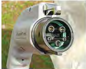
Figure 4: SAE J1772 EV charging plug
