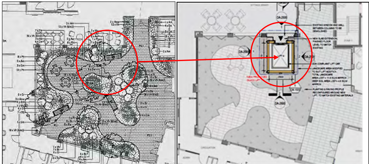
Figure 7 Ground floor plans showing existing central courtyard (left) and proposed lift (right)
