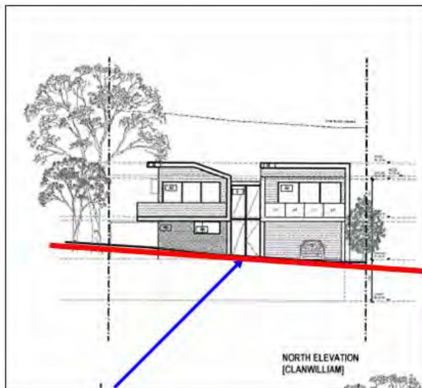
Figure 3: North Elevation - natural ground line at Clanwilliam Street
