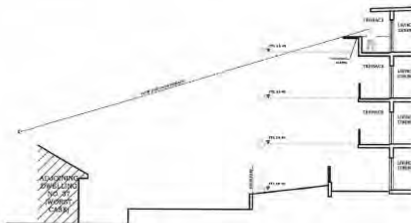
Diagram showing view from balcony with screen louvres in place
