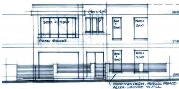
Front elevation – facing Pellisier Road, two storey dwelling with flat roof.
