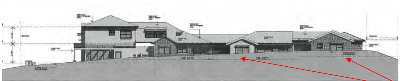
North Elevation showing retention of existing ground level at boundary. Proposed courtyard levels beyond shown dotted
