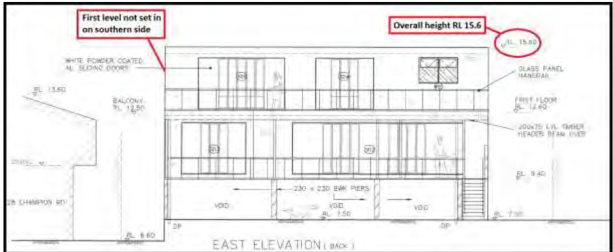
Original Plans – East Elevation, showing original overall height of RL 15.6, and first floor level not set in on southern side.
