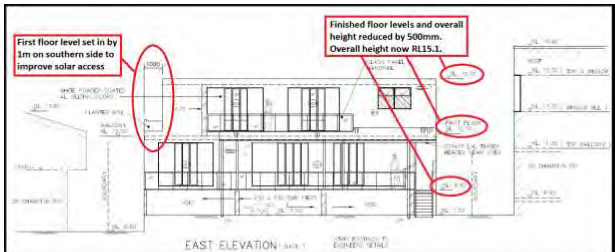
Amended Plans – East elevation, showing first floor level set in by 1m on southern side, and finished floor levels reduced by 500mm.
