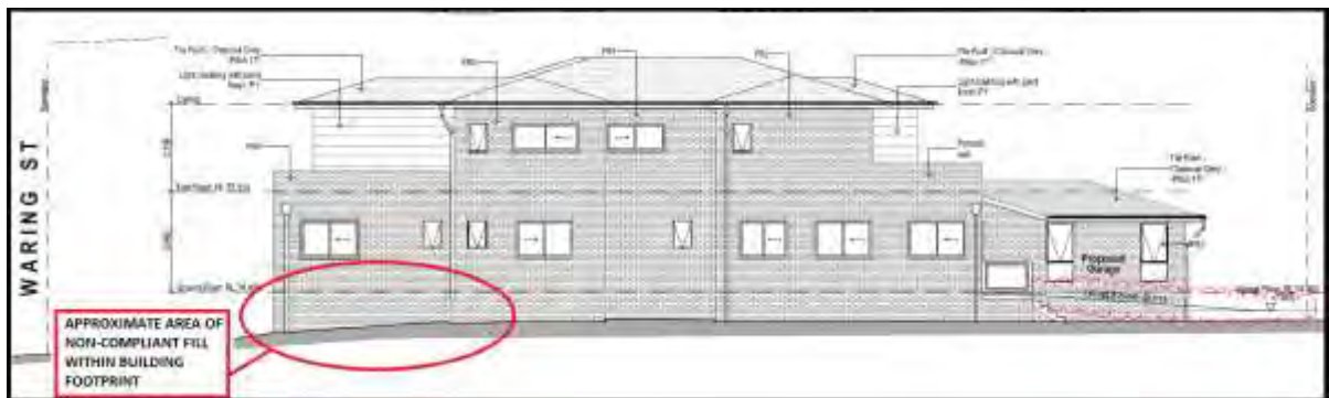
North-west elevation showing area of non-compliant fill within the building footprint. Source: Applicant DA plans, edited.
