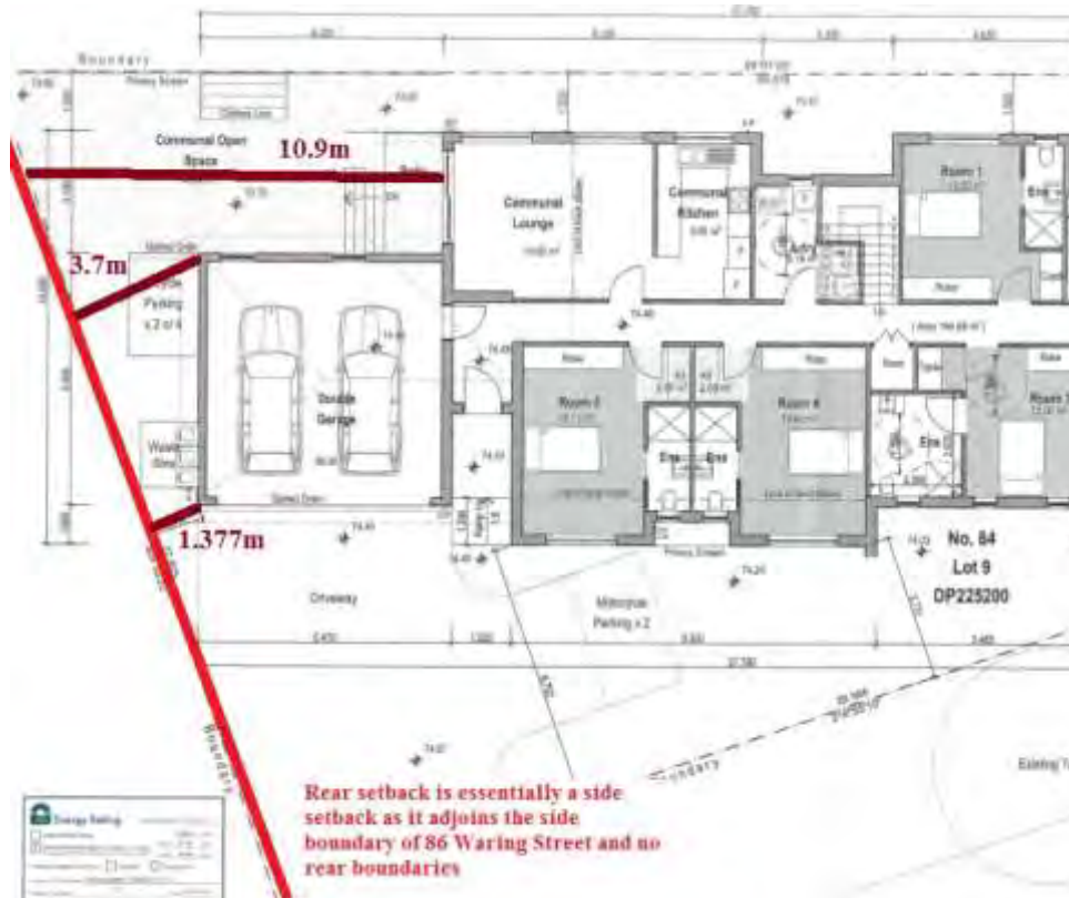
Diagram showing the rear setbacks of the proposed boarding house. Source: Ground Floor Plan by applicant, edited for diagrammatic purposes by CPS
