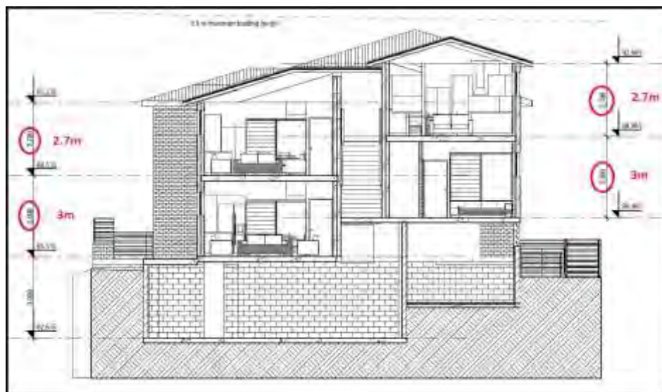
Cross Section of proposed development, showing floor to floor heights. Source: Applicant amended DA plans, marked up.
