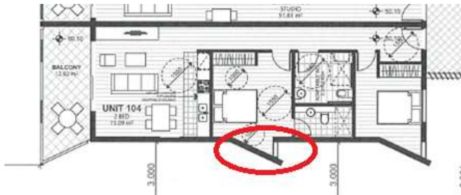
Figure 16: Ear window circled in red. The amendment has deleted the Ear window from the living room and redirect to north facing for bedrooms.
