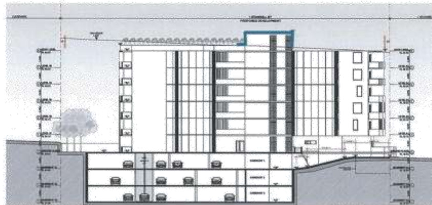
Figure 4.3 | Amended extract of east elevation with the variation of the balustrade and overrun indicated in green
