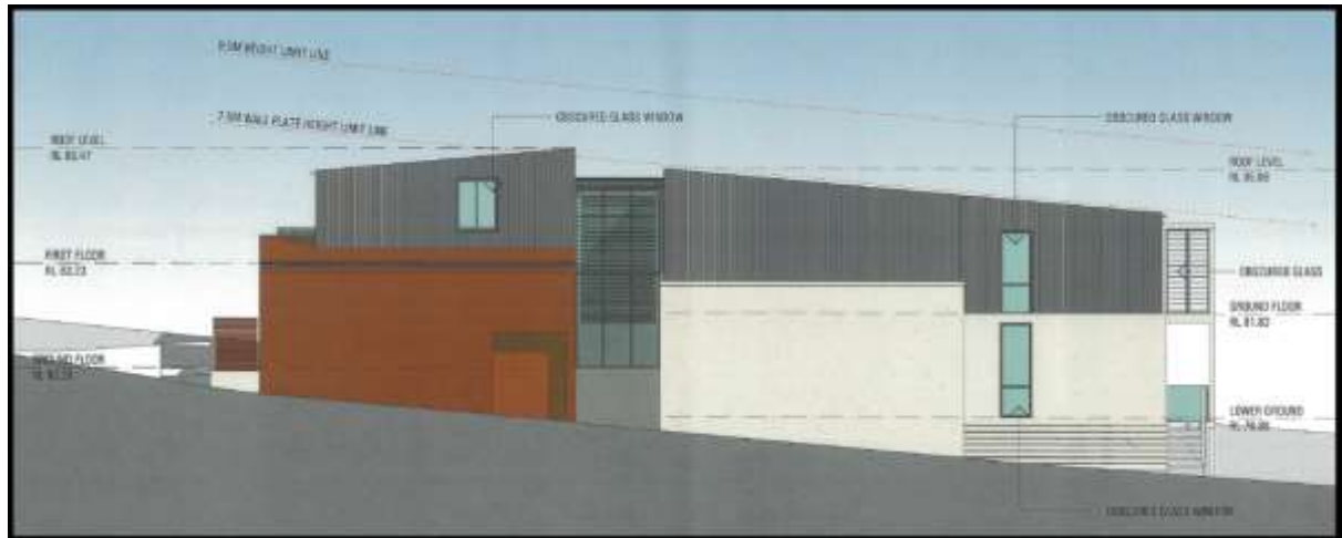
East elevation of proposed development. Note – all windows provided with obscure glass. Source: Applicant DA plans.
