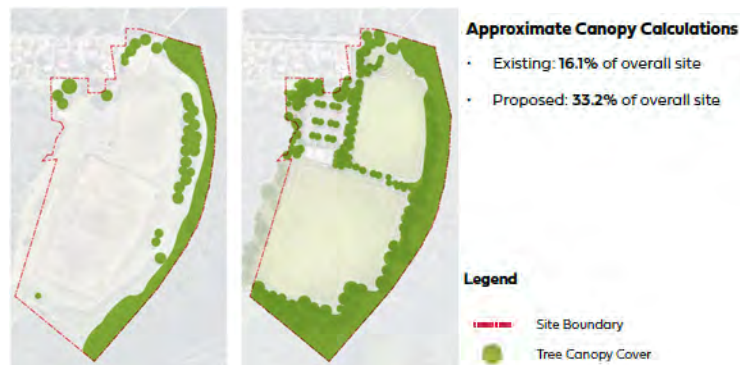
Image 16: Current tree canopy coverage on existing site (16.1%) and Image 17: Increased tree canopy coverage in Masterplan (33.2%), from ATTACHMENT 1
