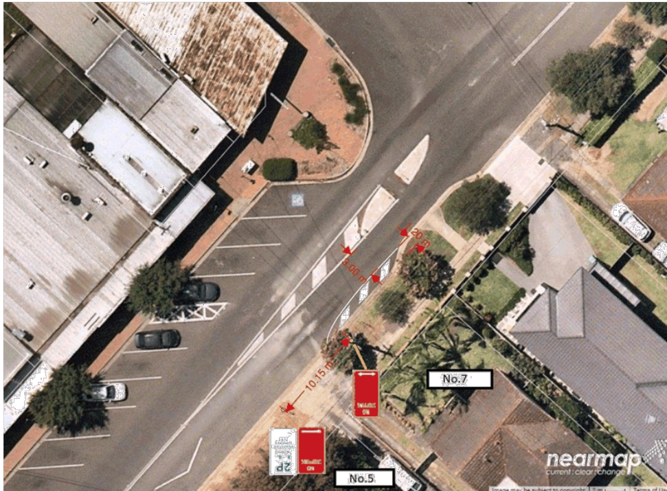
Figure 2: Proposed Extended No Stopping Restrictions and Island.
