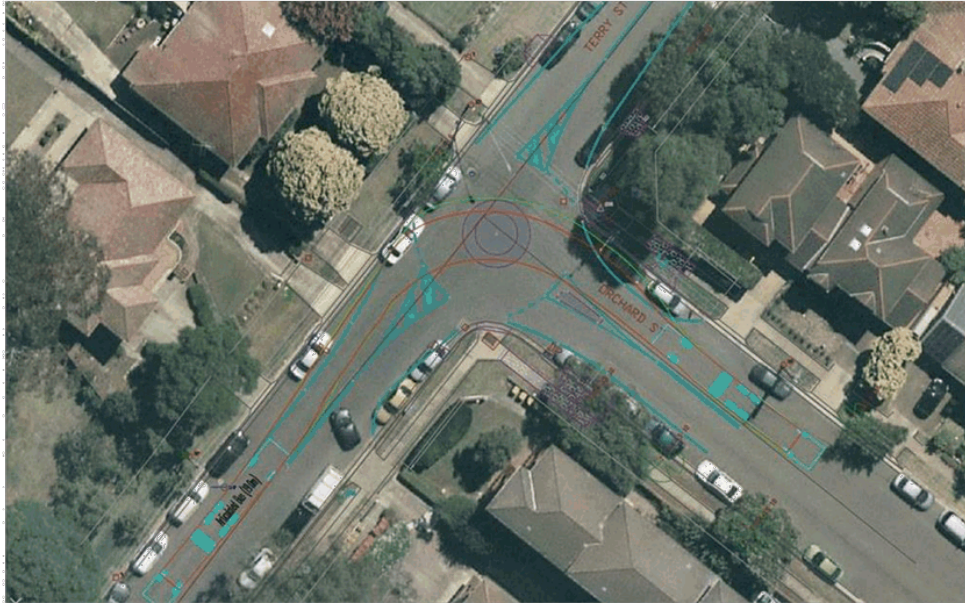
Figure 3: Turning path manoeuvres of rerouted 500X through the roundabout intersection of Terry Road/Orchard Street
