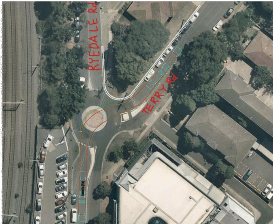
Figure 2: Turning path manoeuvre of rerouted 500X through the roundabout intersection of Ryedale Road/Terry Road
