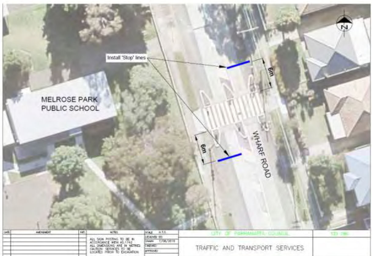
Figure 5: Upgrade of existing pedestrian crossing to become a combined children & pedestrian crossing
