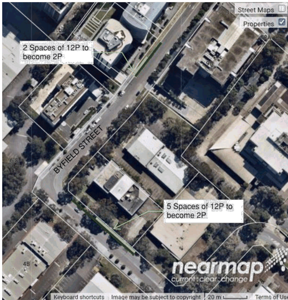
Figure 3: Byfield Street – Recommendation C
