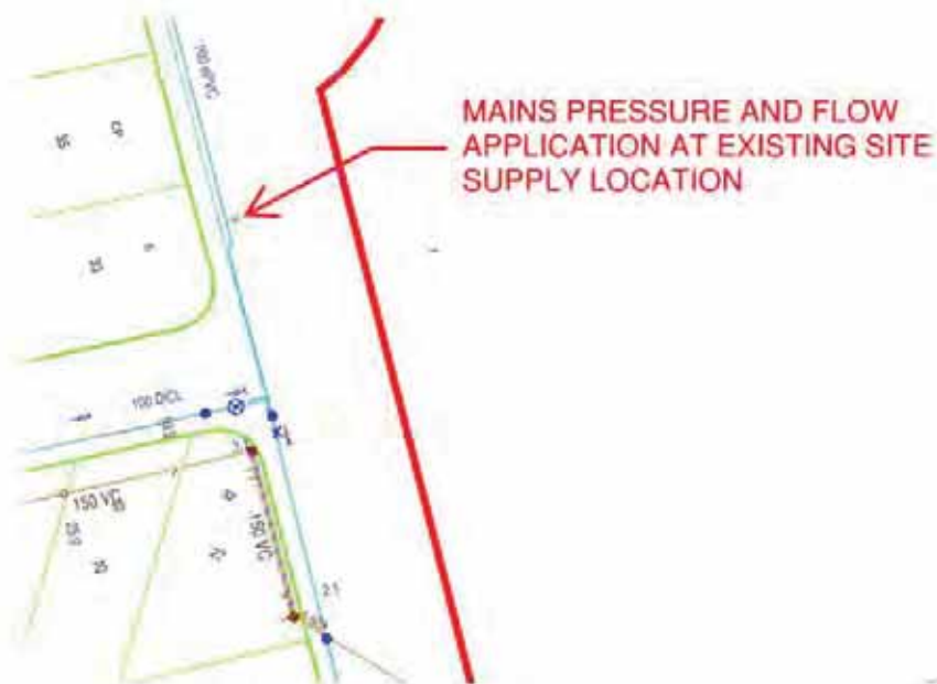
Figure 6: Mains locations of water pressure and flow test
