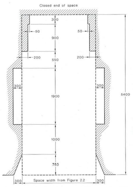
NOTE: The design envelope provides for structural elements to be clear of all four side doors.
