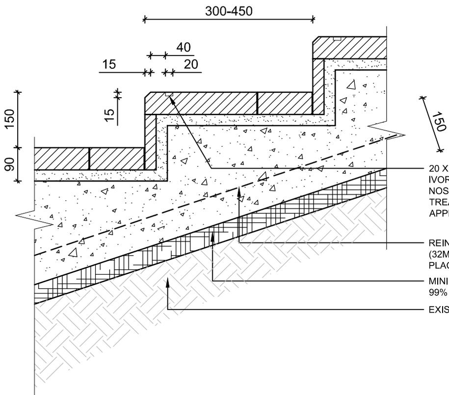
20 X 10 SAFETY STAIR BAR. ALUM. CLAD IVORY SILICON CARBIDE SETBACK 40 FROM NOSING TO FULL LENGTH OF EACH STAIR TREAD. CONTRASTING COLOUR TO BE APPROVED BY LANDSCAPE ARCHITECT
