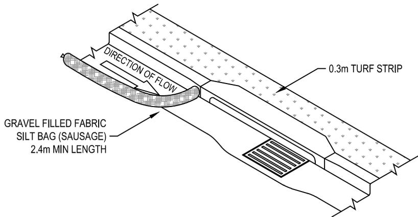
**KERB INLET SEDIMENT TRAP**
