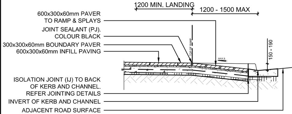
**PV 4.6a** KERB RAMP - SECTION
