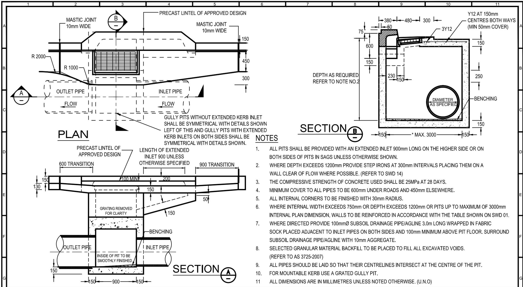
GULLY PITS WITHOUT EXTENDED KERB INLET SHALL BE SYMMETRICAL WITH DETAILS SHOWN LEFT OF THIS AND GULLY PITS WITH EXTENDED KERB INLETS ON BOTH SIDES SHALL BE SYMMETRICAL WITH DETAILS SHOWN.
