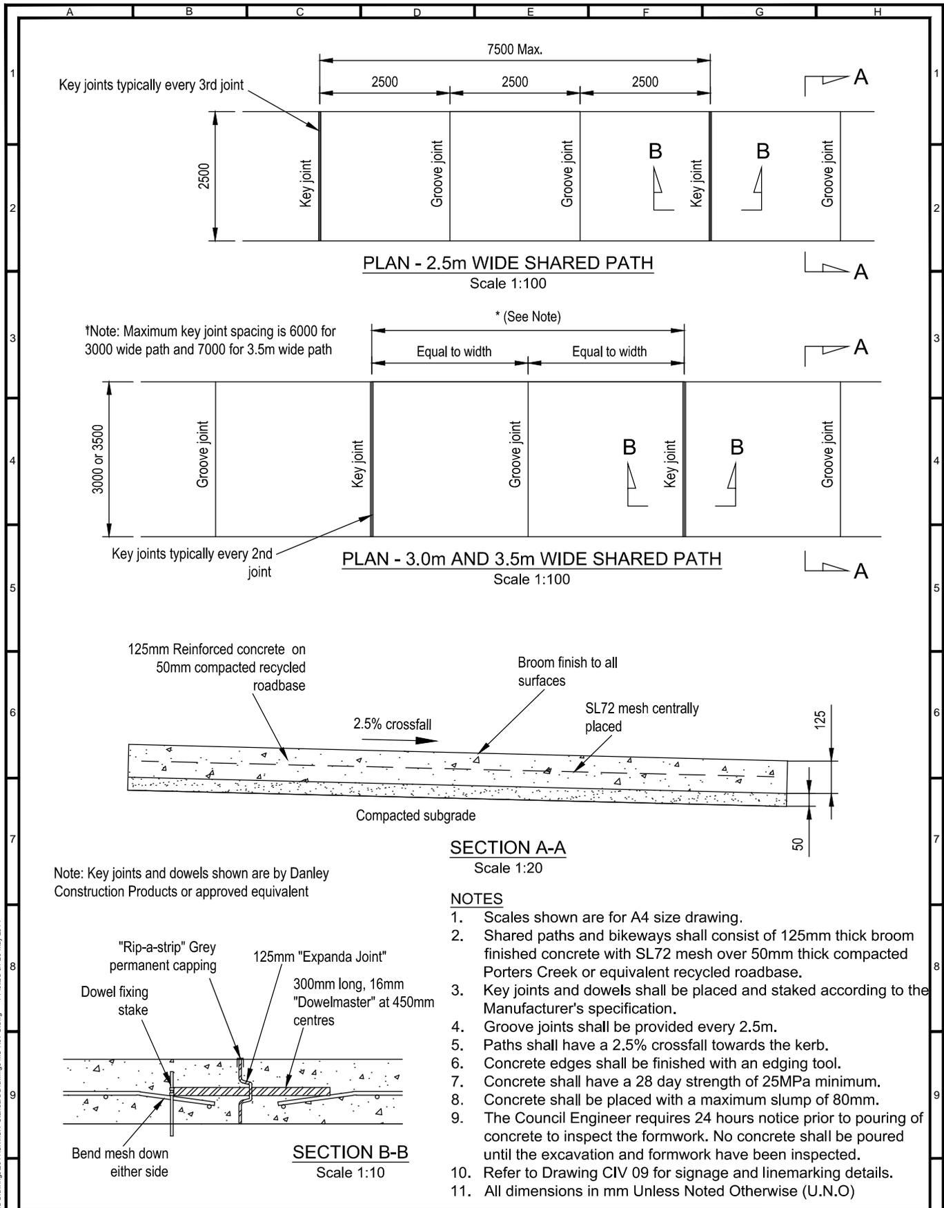
Note: Key joints and dowels shown are by Danley Construction Products or approved equivalent
