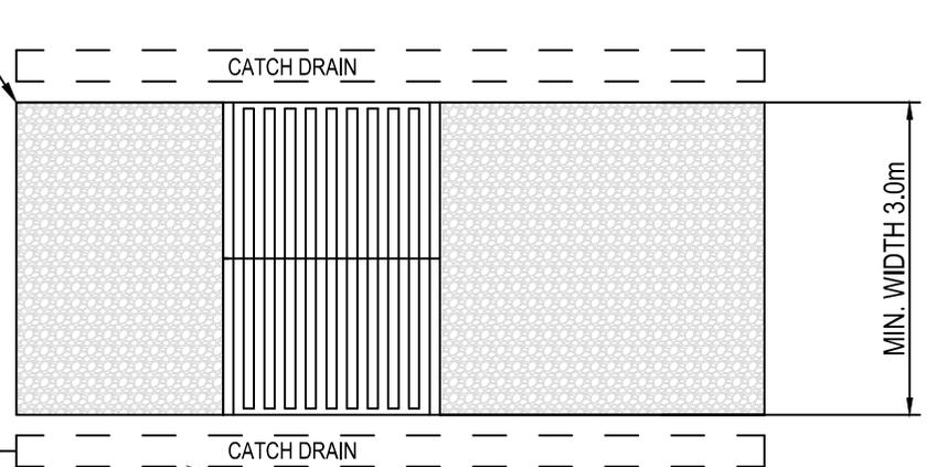
RUNOFF FROM GRIDS TO BE DIRECTED TO SEDIMENT TRAP.
