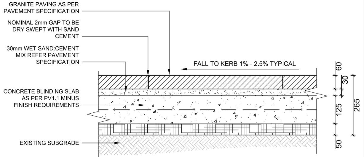
**PV 1.2 PAVEMENT TYPE GRANITE - TYPICAL**
