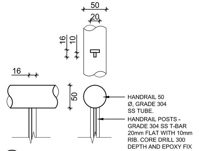
**HR 1.3** POST TO HANDRAIL - PLAN & SECTION
