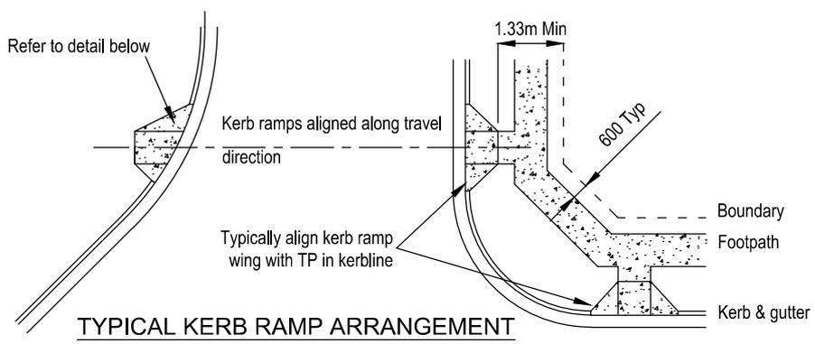
**TYPICAL KERB RAMP ARRANGEMENT AT INTERSECTIONS**
