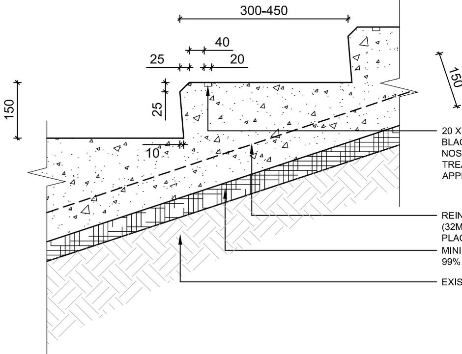
20 X 10 SAFETY STAIR BAR. ALUM. CLAD BLACK SILICON CARBIDE SETBACK 40 FROM NOSING TO FULL LENGTH OF EACH STAIR TREAD. CONTRASTING COLOUR TO BE APPROVED BY LANDSCAPE ARCHITECT
