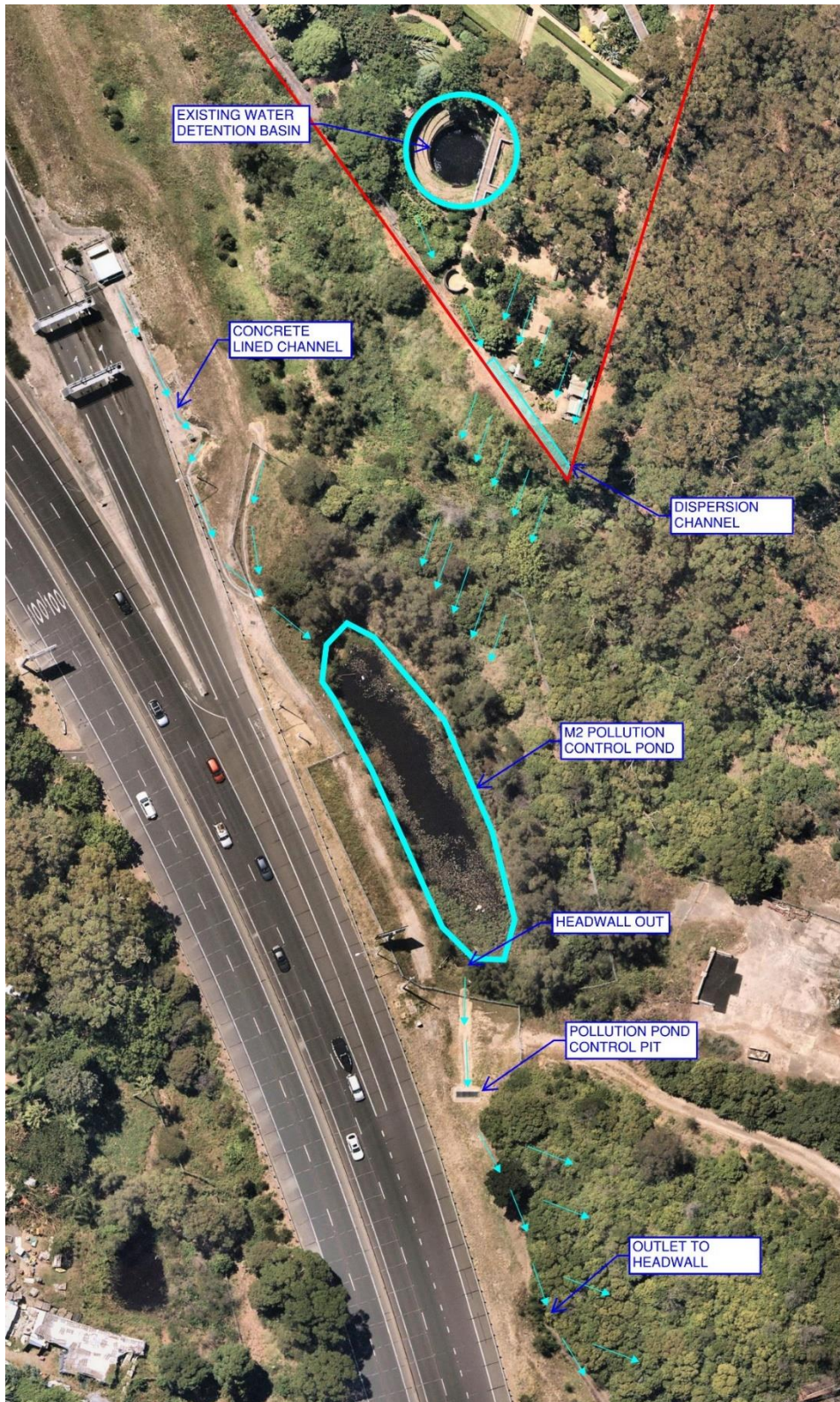
Figure 7: Downstream of Site - M2 Ancillary Drainage Structures
