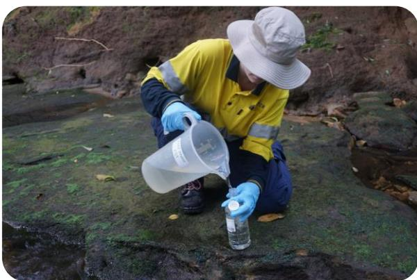
Figure 6 Collecting water samples for analysis
