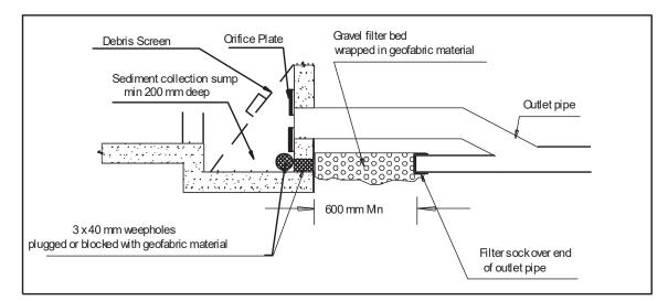
SEDIMENT COLLECTION SUMP WITH DRAINAGE FILTER TYPICAL DETAIL OF AN OUTLET CONTROL PIT/SUMP WITH SIDE DRAINING SEDIMENT COLLECTION SUMP Note the filter medium between the weepholes and the connection to the outlet pipeline
