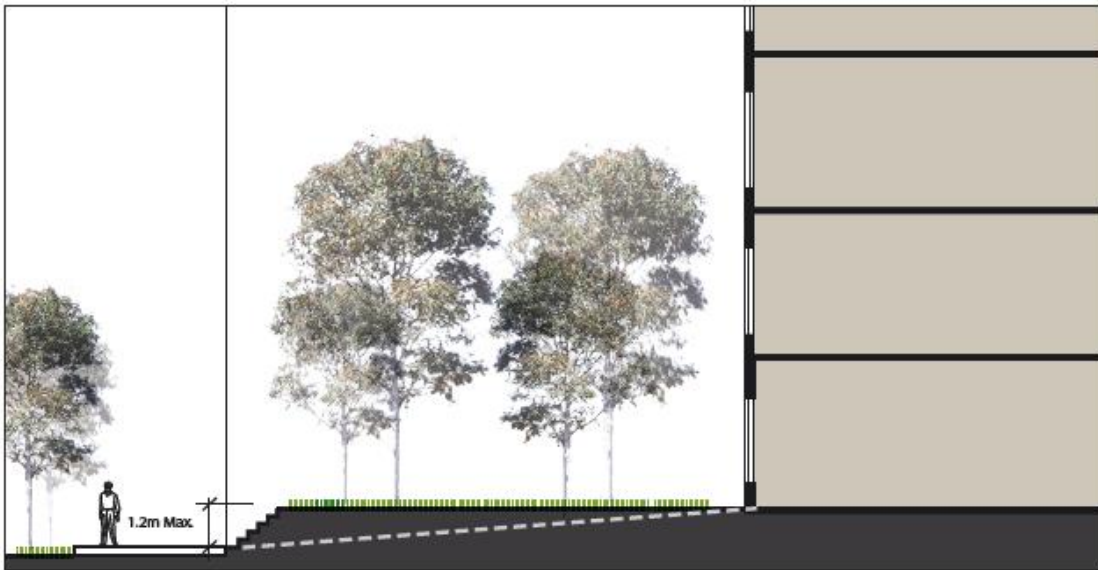
Figure 8.4.3 Level change controls where publicly accessible open space is located adjacent to a street.
