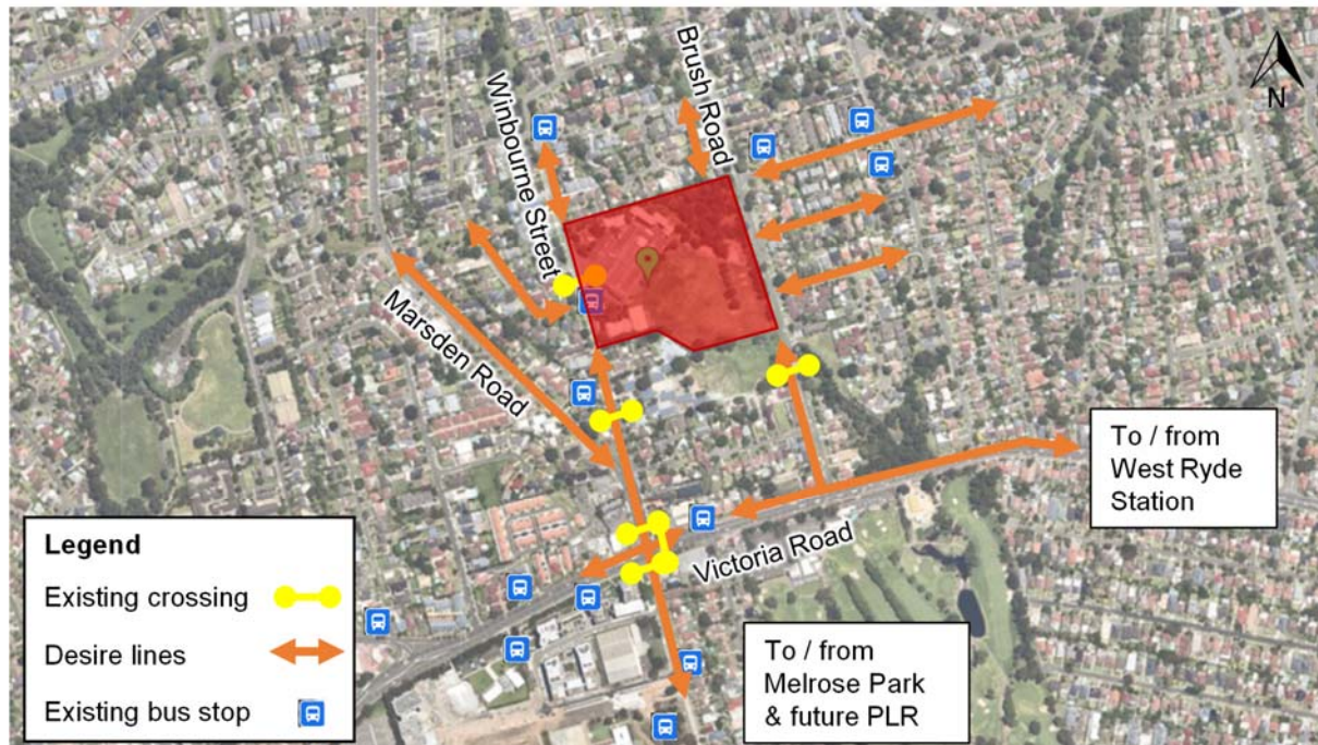
Figure 6.1: Pedestrian Desire Lines and Existing Crossings
