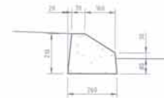
MOUNTABLE KERB (MK) SCALE 1:10
