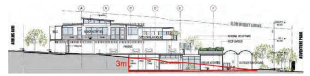
Figure 19: Extract from the Section A-A Plan showing the extent of excavation in red.
