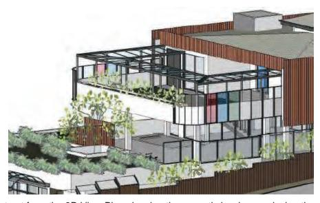
**Figure 17**: Extract from the 3D View Plan showing the acoustic barriers enclosing the side of the first floor balcony. The acoustic barrier is also required to enclose the rear side of the balcony (not shown in this image).
