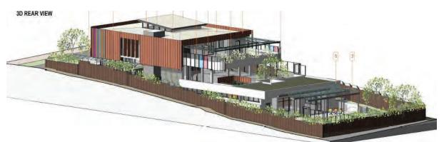
**Figure 24**: Extract from the Applicant's 3D View Plan showing the scale of the overall development including the boundary fencing / acoustic barriers. The acoustic barrier is also required to enclose the rear side of the first floor balcony (not shown in this image).
