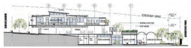
**Figure 15:** The Section Plan showing the extent of excavation for the Lower Ground Level. The development satisfies the maximum permitted height of buildings as shown by the 9.5m height limit line.
