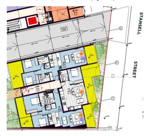
**Figure 22 –** Extract of ground floor plan showing private open space areas of units G.01, G.02 and G.03 in yellow highlight The composition of the private open space areas for these units are as follows:
