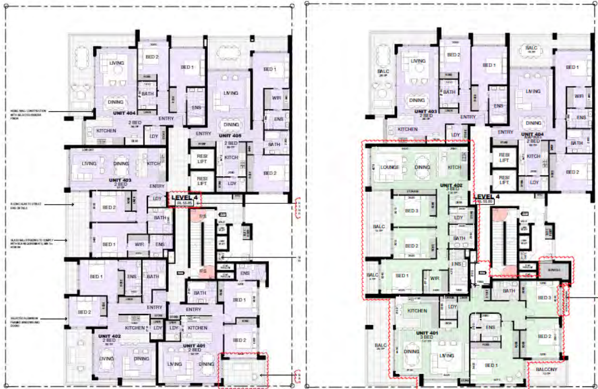
Figure 7 – Level 4 floor plans comparing originally approved on the left and proposed to the right
