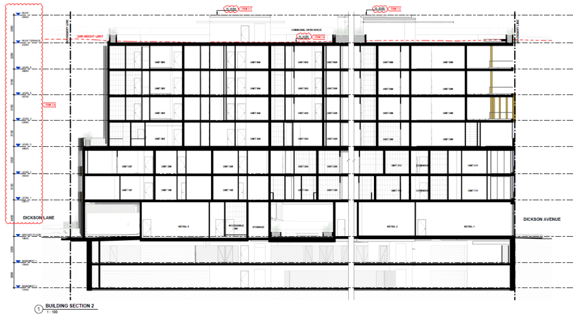
Figure 11 – Proposed Section Plan showing the 24m maximum building height as red dashed line
