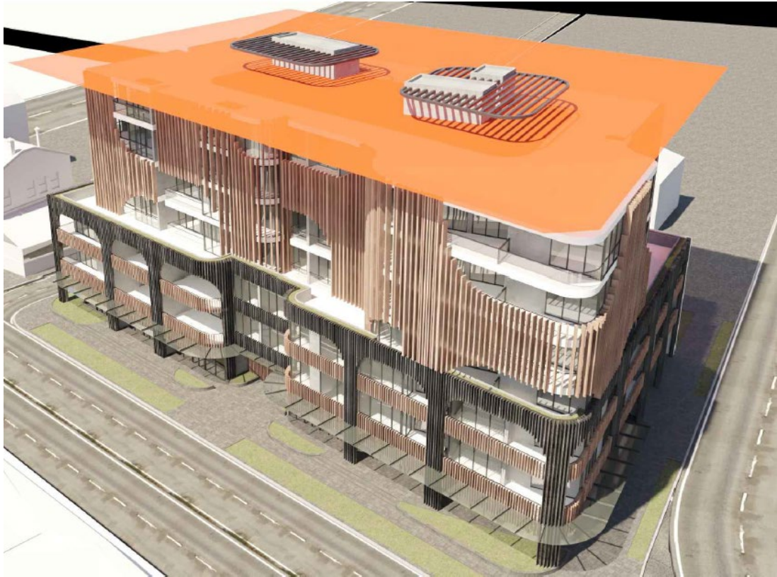
Figure 8 – Approved 24m Building Height Plane shown in orange.
