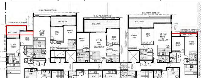
Figure 23: Illustration of the non compliance with building depth on the northern and southern boundary. The area outlined in red is the area of non compliance being 2.2m along the southern boundary and 0.6m along the northern boundary.
