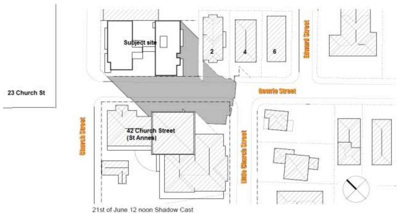
Figure 14: Shadow diagram at 12 noon 21 st June.
