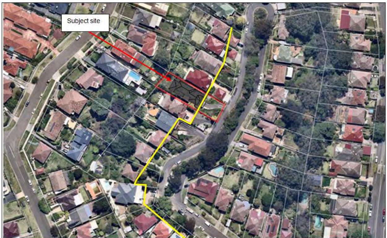
Figure 19 – Indicative aerial photograph with the roof of the proposed superimposed on existing (new roof colour is charcoal for No 35 Buena Vista Avenue). Black lines indicate the main ridge lines of the proposed and yellow line indicates the established building line.
