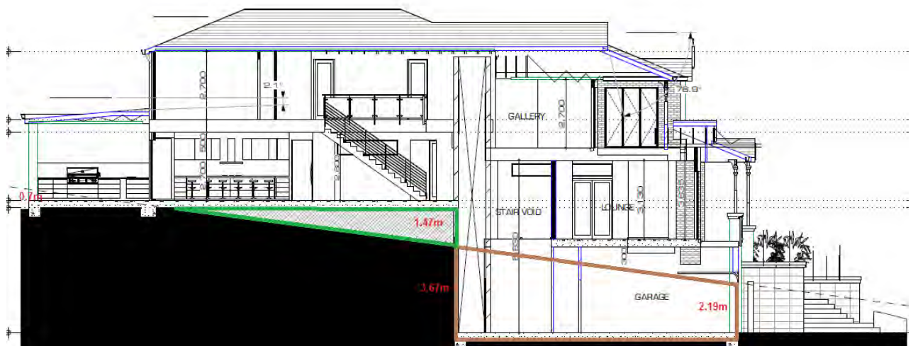
Figure 15 – Locations of cut (brown) and fill (green).
