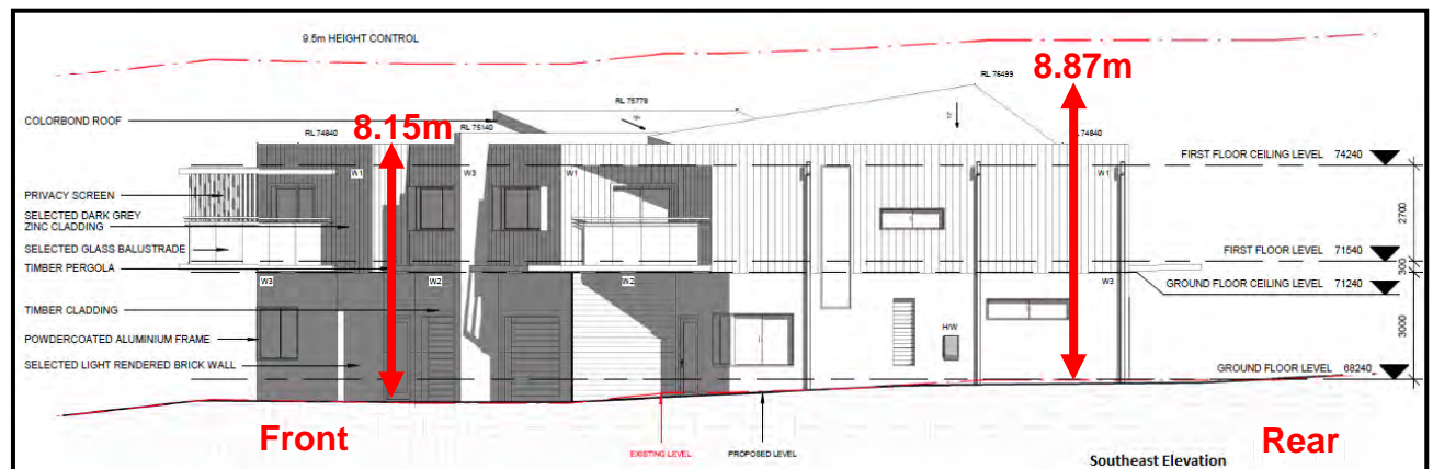
Figure 10: Southeast elevation demonstrating proposed dual occupancy will be under the 9.5m max building height (Source: ARC Homes)
