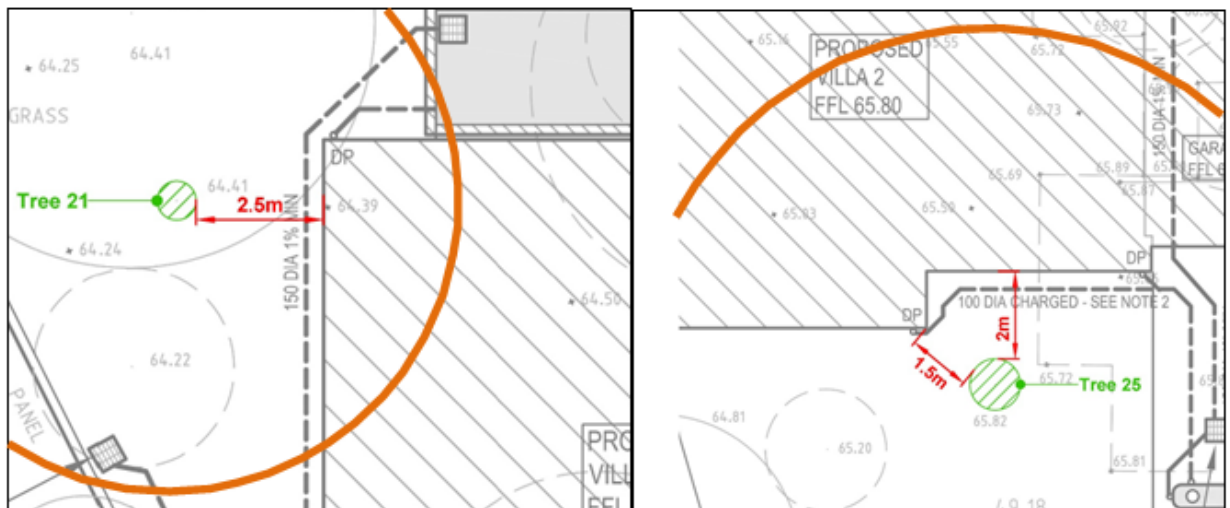
Figure 15: Proximity of enclosed walls and stormwater infrastructure in relation to T21 and T25
