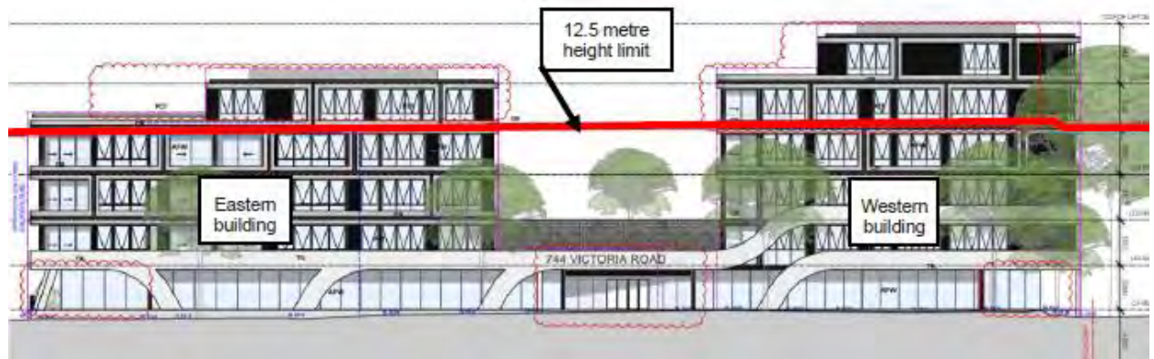
Figure 21: North elevation showing extent of building exceeding 12.5m building height
