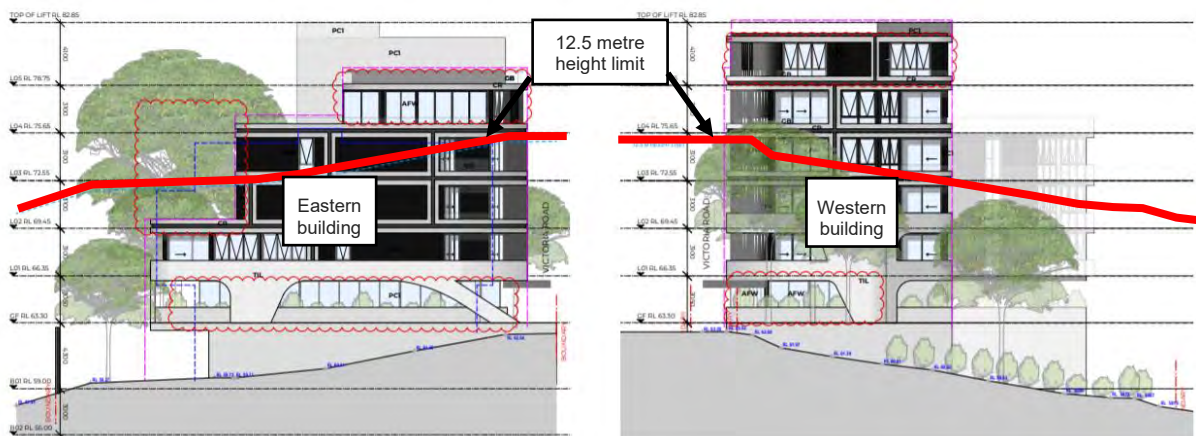
Figure 3: East (left) and West (right) Elevations (Source: Aleksandar Projects)
