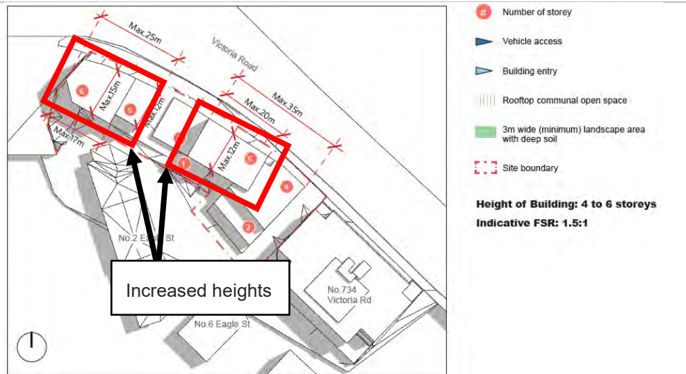
Figure 5: Building scale (Source: Ryde City Council)
