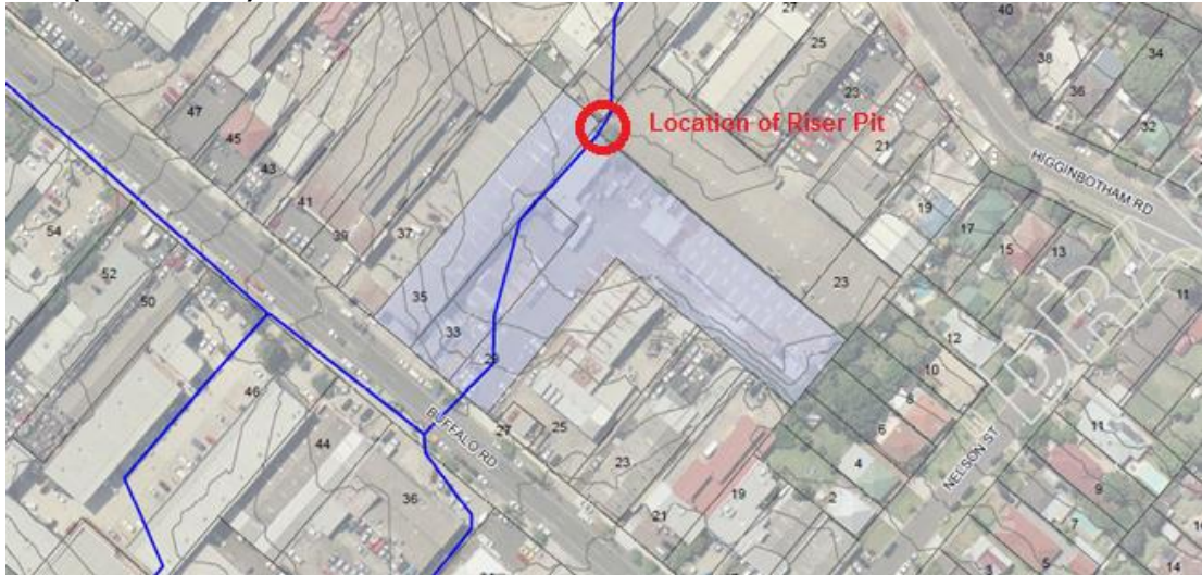
Figure 8: Location of the existing 1,050mm diameter stormwater pipe and the Council owned riser pit (circled).
