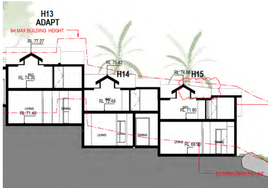
Figure 20: Extract from Section AA showing the 'existing ground line' in relation to Dwellings H13 – H15
