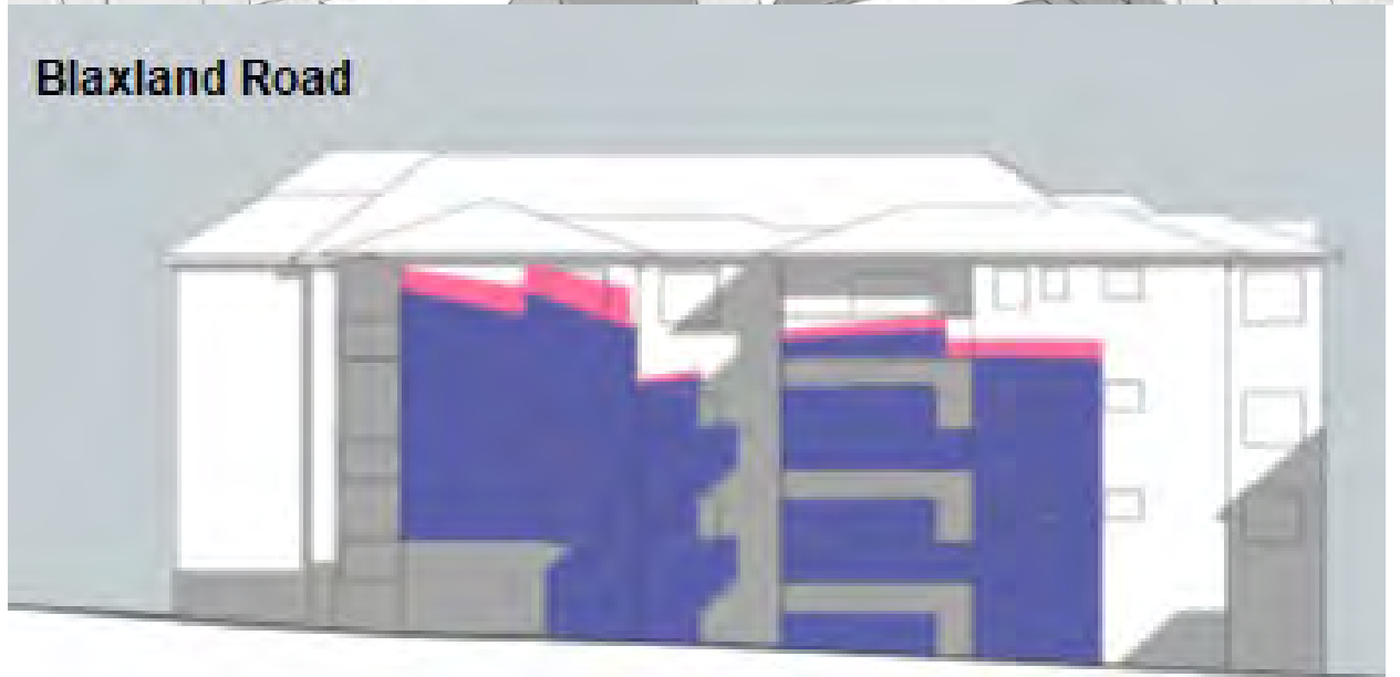
Figure 19: 3pm – blue illustrate shadow generated from compliant height. Pink illustrate the additional shadow generate by the additional height on the adjoining southern property.
