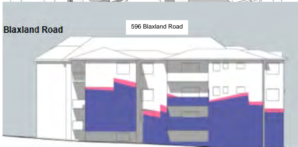
Figure 18: 12 noon – blue illustrate shadow generated from compliant height. Pink illustrate the additional shadow generate by the additional height on the adjoining southern property.
