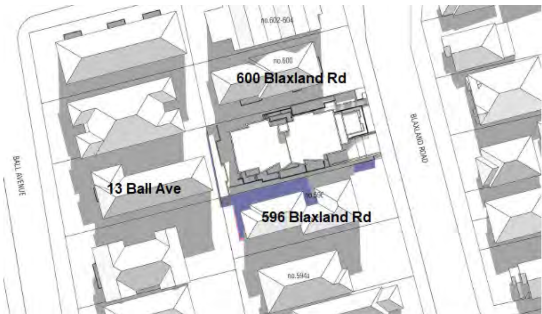
Figure 29: Overshadowing to adjoining properties at 9am on 21 June.
