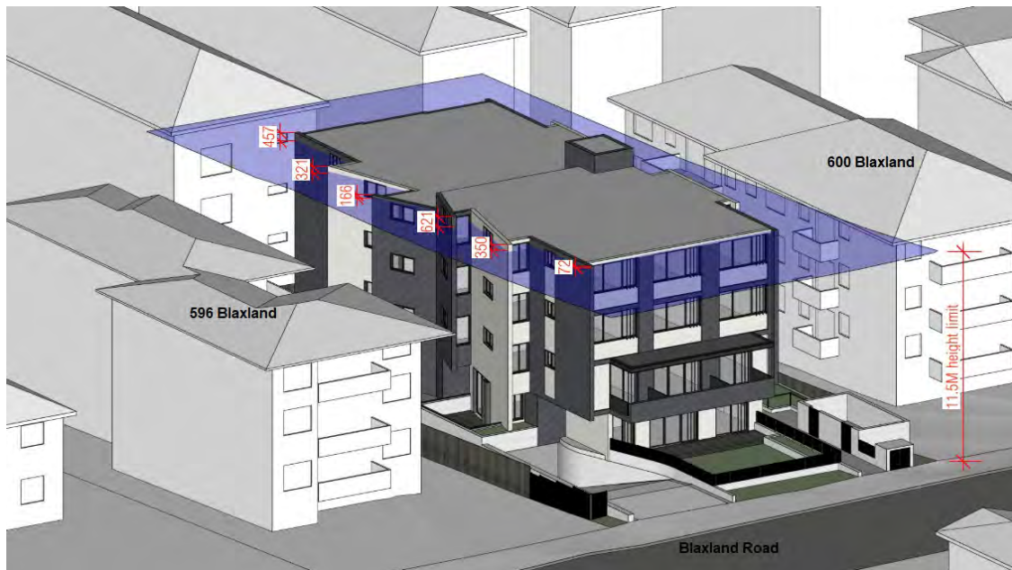
Figure 12: South east view – the section above the purple plane is the area where it breaches the height plane.
