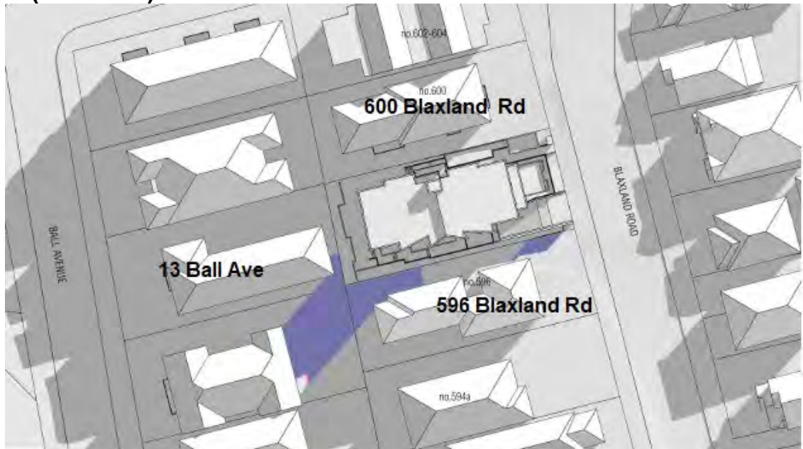
Figure 29: Overshadowing to adjoining properties at 9am on 21 June.
