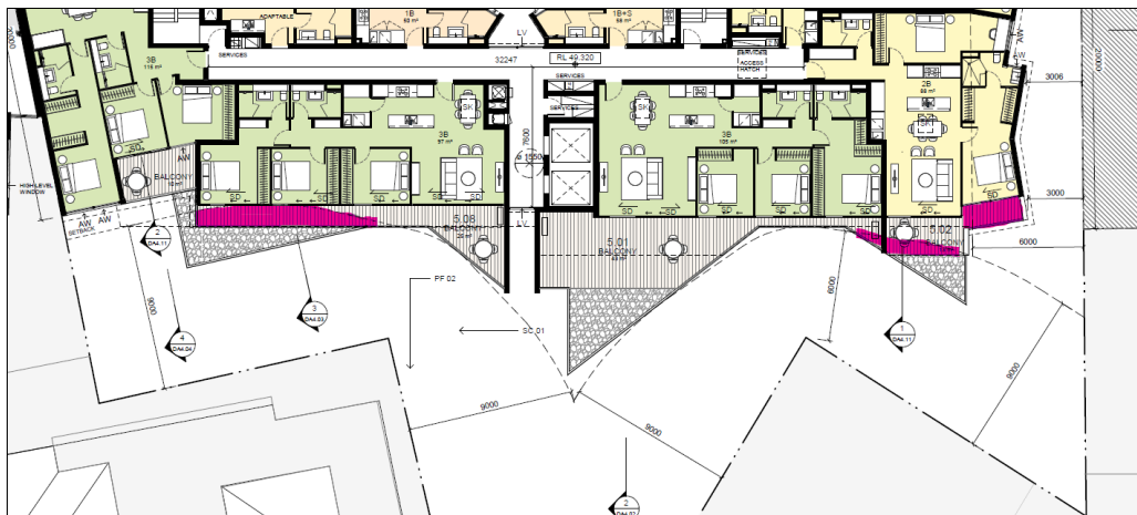
Figure 24 Balconies which encroach within the required separation distance
