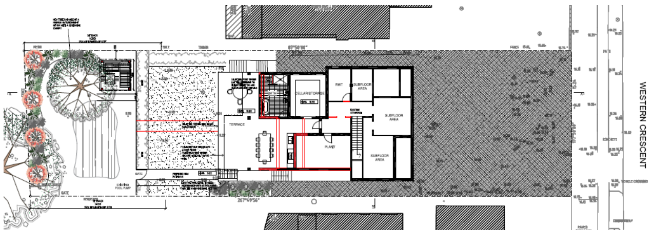
Figure 8 - Proposed Lower Ground Floor Plan (existing walls shown in black and proposed in red)
