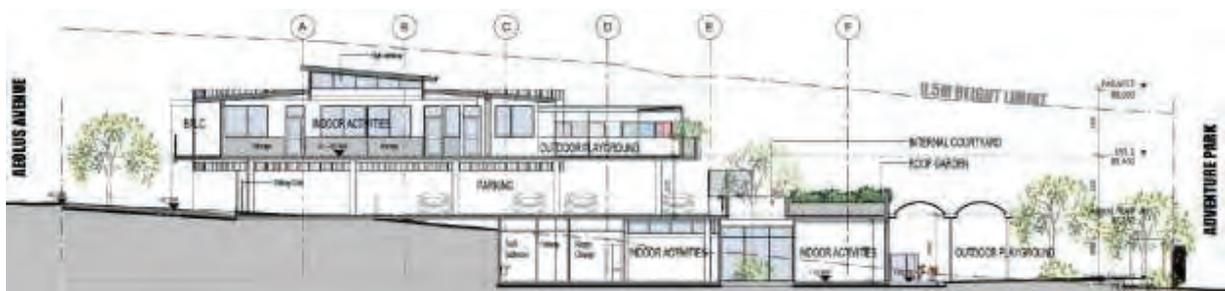
**Figure 15:** The Section Plan showing the extent of excavation for the Lower Ground Level. The development satisfies the maximum permitted height of buildings as shown by the 9.5m height limit line.
