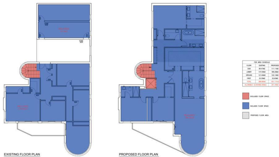
**Figure D: Lower Ground Floor Plans – existing and proposed – showing changes to floor layout and area of additional GFA**
