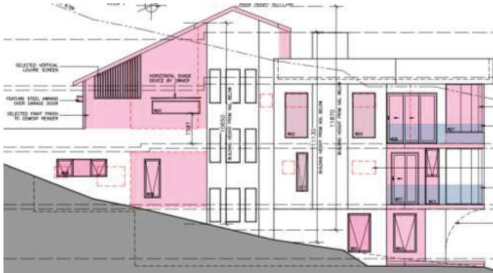
The additions will also create a continuous building height measured at 10.65m, although “ground level (existing)” would be unchanged by this aspect.
