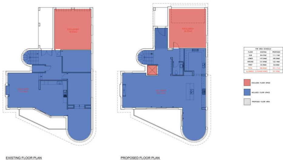
**Figure E: Ground Floor Plans – existing and proposed – showing changes to floor layout and area of additional GFA**
