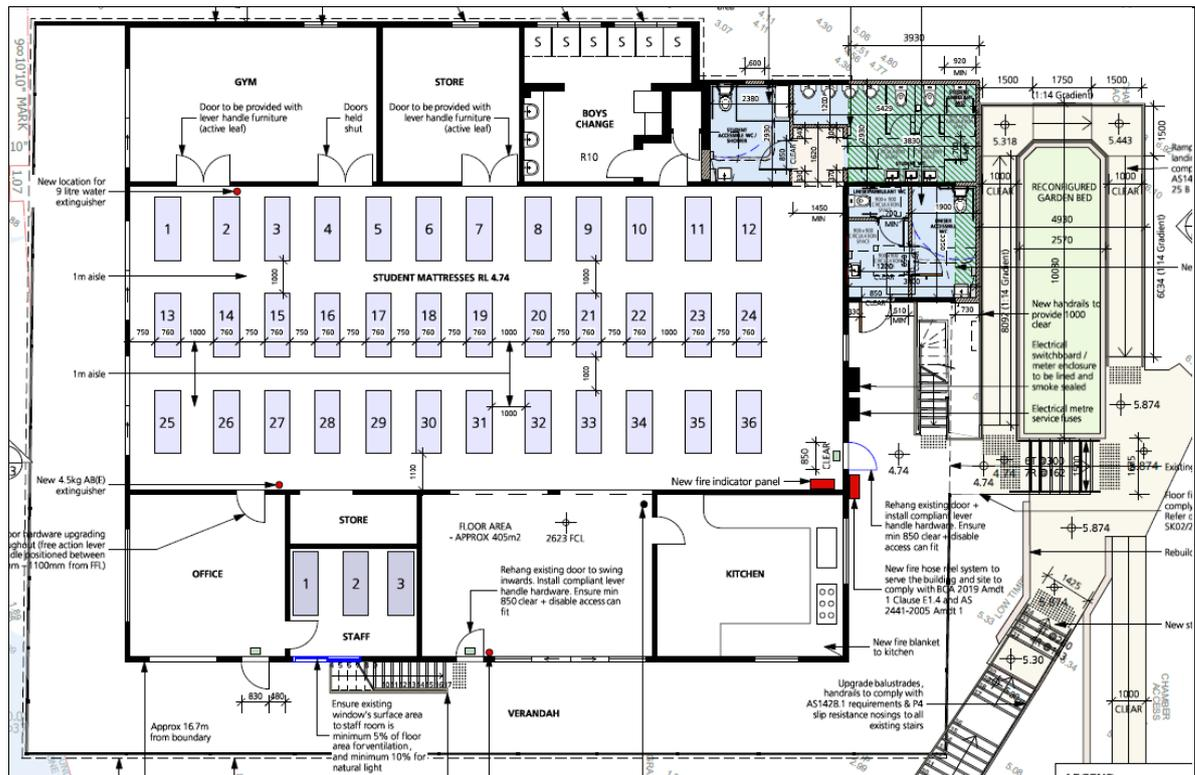
Figure 7 – Extract of proposed first floor plan depicting layout of student mattresses
