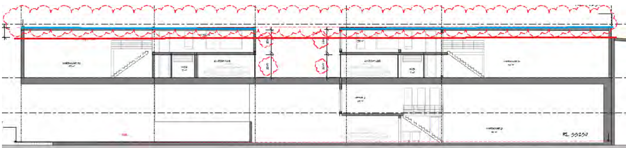
Figure 26 Extent of height breach (roof height in blue and red line depicting 10m height line) parallel to the lowest RL on the site
