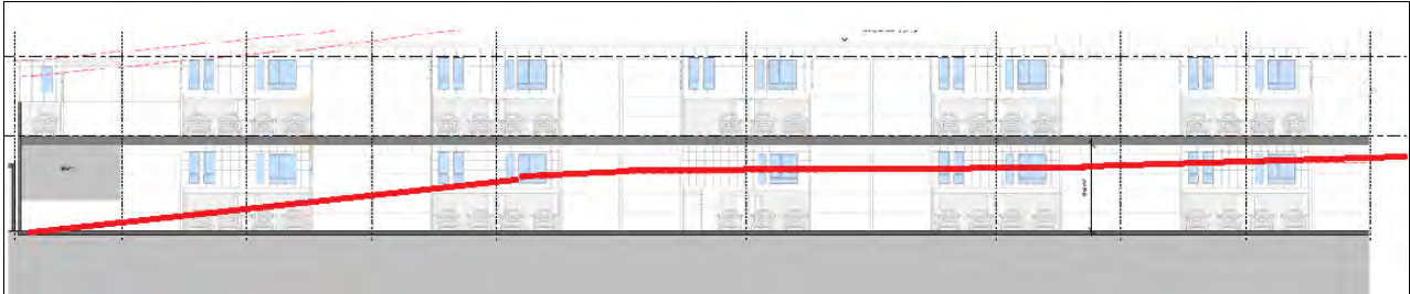
Figure 19 Natural ground level shown in red from Warehouse 18 – 9 (basement floor) and Warehouse 42 – 32 (ground floor) to rear of the site along south eastern elevation
