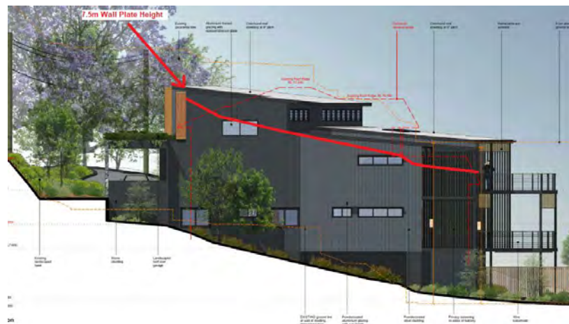
Figure 17 - Wall Plate Height Non-Compliance (North Elevation)
