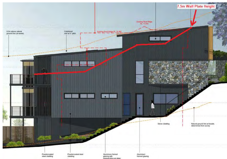
Figure 16 - Wall Plate Height Non-Compliance (South Elevation)
