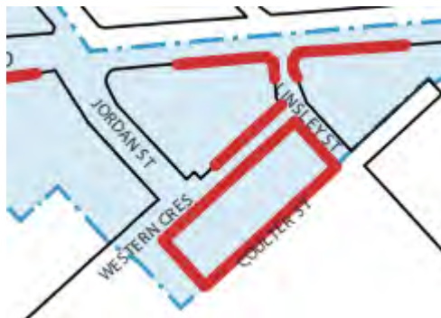
Figure 27 – Extract of Buildings Abutting the Street Alignment Control Drawing (buildings required to abut the street alignment where red lines located)
