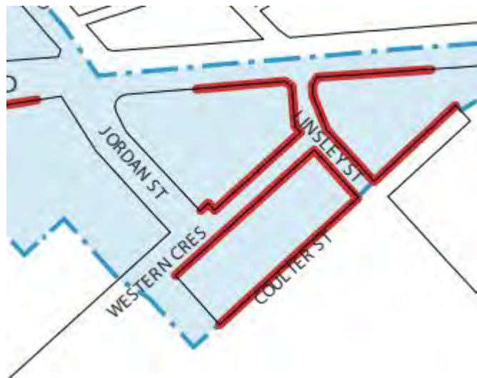
Figure 33 – Extract from DCP Awnings Control Drawing (requirement for awnings denoted by red lines)
