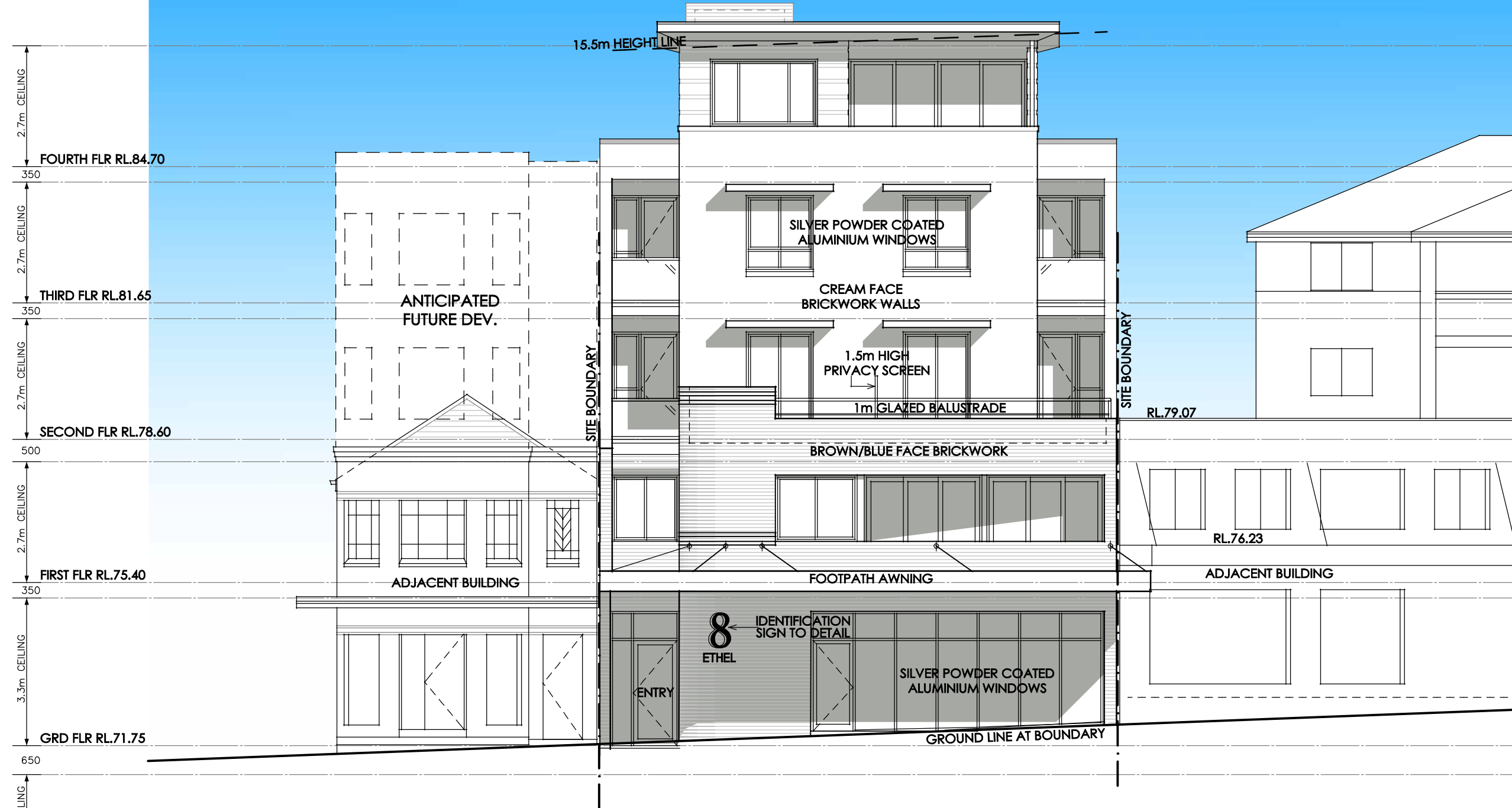
SOUTH (ETHEL ST) ELEVATION SCALE 1:100
