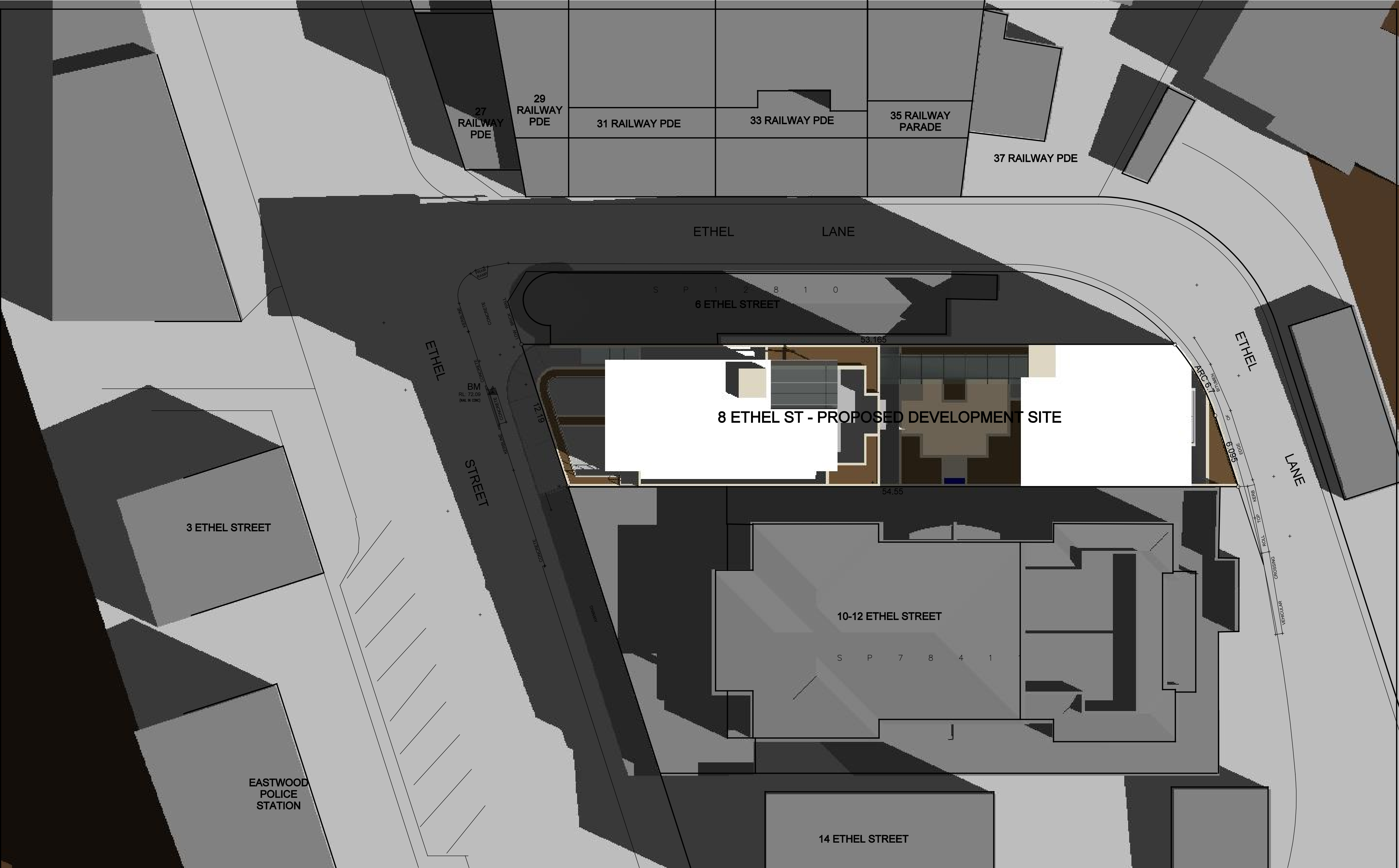
SHADOW DIAGRAM: 22 JUNE - 10AM SCALE 1:200
