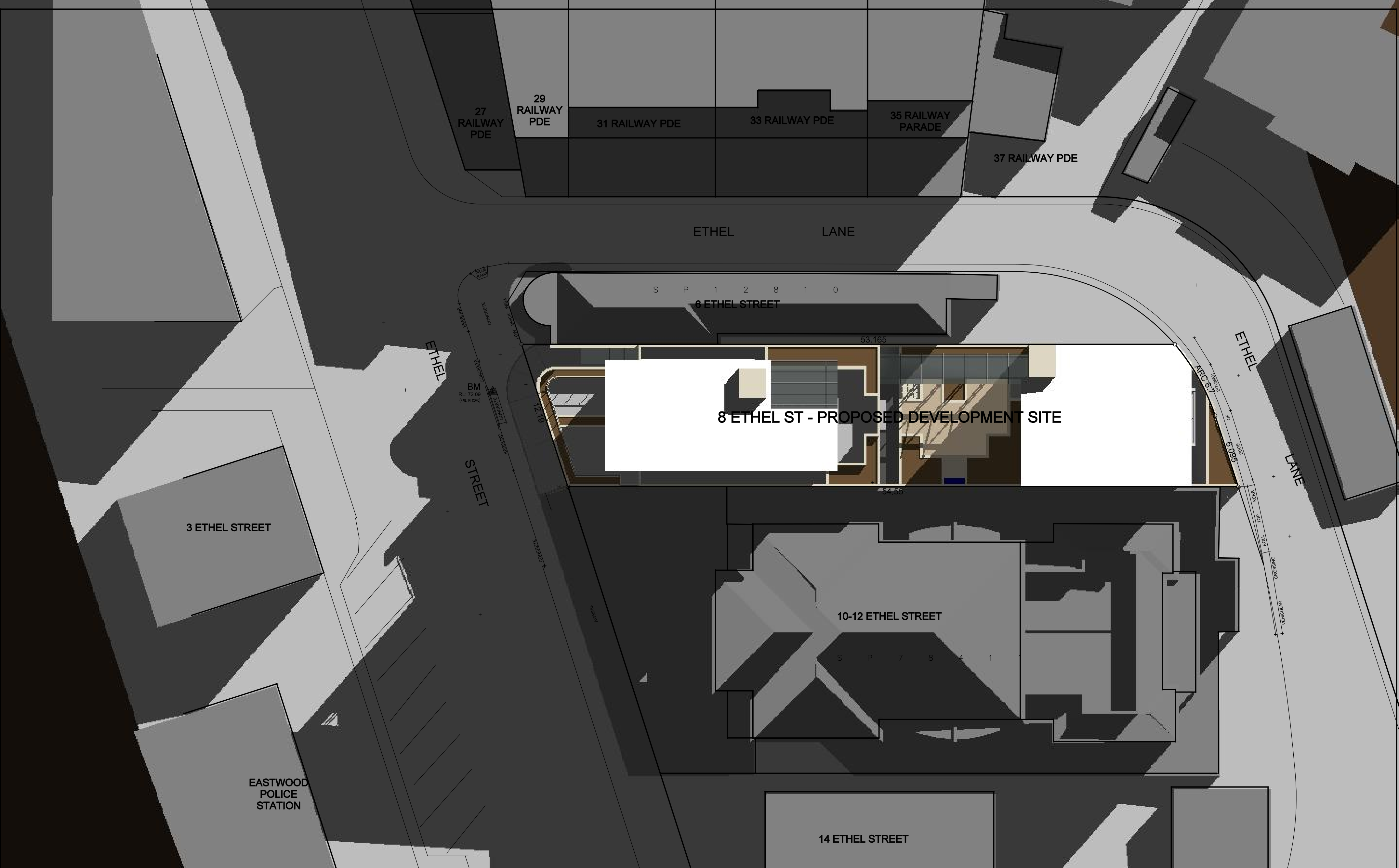
SHADOW DIAGRAM: 22 JUNE - 3PM SCALE 1:200
