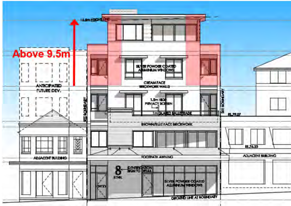
Figure 15: Extract of the South (front) Elevation Plan showing the portions of the upper levels which do not satisfy the minimum 3m side setbacks in the DCP (shaded in red).
