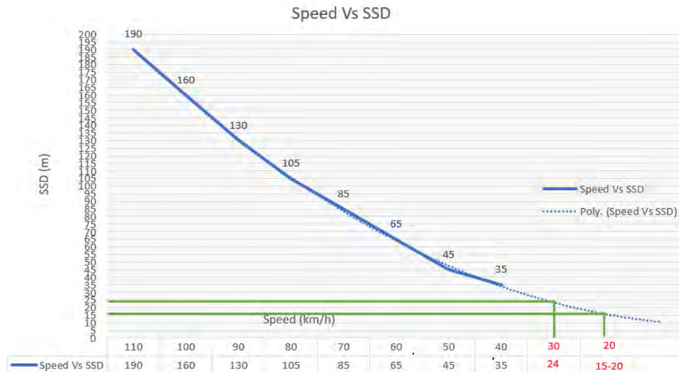
Figure 26: Figure 3.2 of AS2890.1 showing the extrapolated stopping distance of 15-20m for vehicles travelling less than 40km/h.
