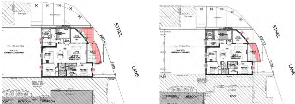
Figure 17: Extracts from the Second (left) and Third (right) floor plans showing the portions of these upper levels which do not satisfy the minimum 3m rear setback in the DCP (shaded in red).
