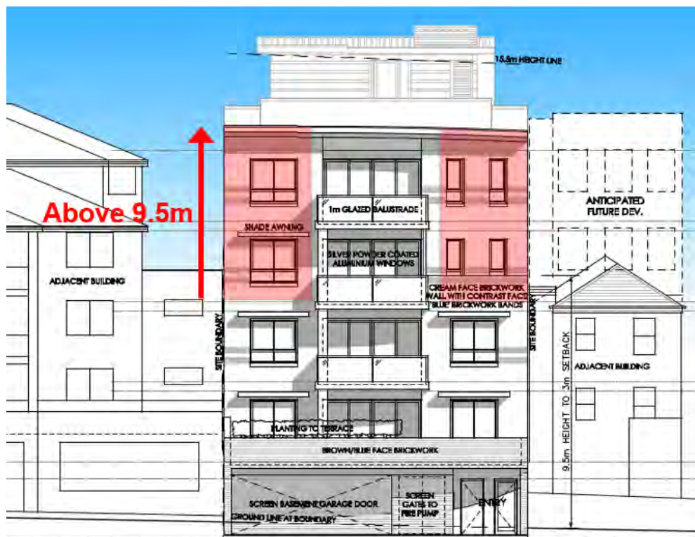
Figure 16: Extract of the North (rear) Elevation Plan showing the portions of the upper levels which do not satisfy the minimum 3m side setbacks in the DCP (shaded in red).
