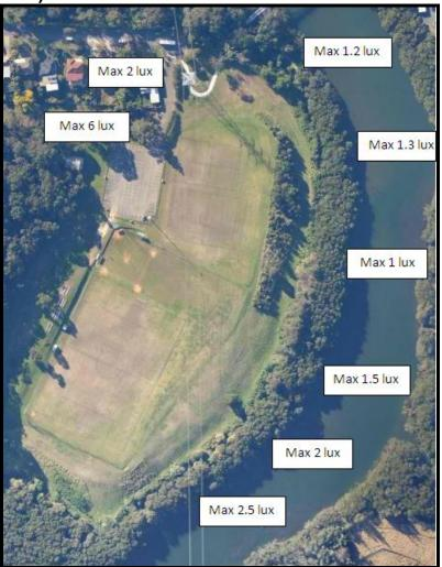
Figure 5: Light level measurements as a result of the proposed Section 96 Modification
