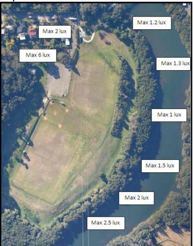
Figure 3: Light level measurements as a result of the proposed Section 96 Modification
