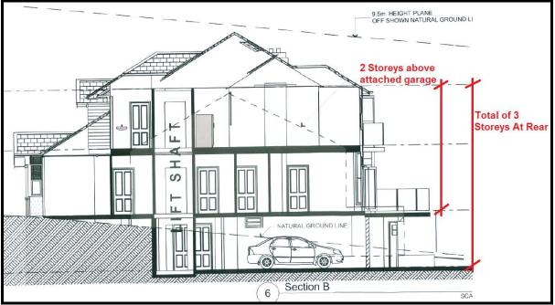
**Figure 2** – Section demonstrating three (3) storey component of dwelling at the rear with two (2) storeys located above the attached garage.
